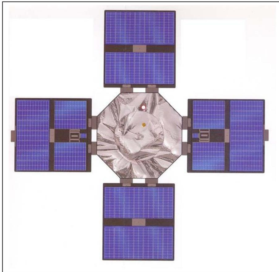
NASA's twin Van Allen Probes spacecraft will be launched in 2012. The figure above shows the octagonal spacecraft body and the location of the surrounding four solar panel 'wings' that provide power to the spacecraft instruments. The small blue rectangles within each of the four solar panels show the location of the solar cells used to power the satellite. As the spacecraft orbits Earth, the four solar panels continuously face the sun to provide constant power.
