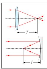
Any optical system, such as a telescope, camera or microscope, can be described by a just few basic numbers.
