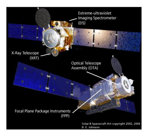
The Hinode satellite weighs approximately 700 kg (dry) and carries 170 kg of gas for its steering thrusters, which help to maintain the satellite in a polar, sun-synchronous orbit for up to two years. The satellite has two solar panels (blue) that produce all of the spacecraft's power. The panels are 4 meters long and 1 meter wide, and are covered on both sides by solar cells.
