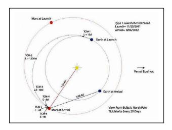
The Mars Science Laboratory was launched from Cape Canaveral on November 26, 2011 for a 251-day journey to Mars along an orbital path 567 million kilometers in length. The path is along a portion of an elliptical orbit called a Hohmann Transfer Orbit.
