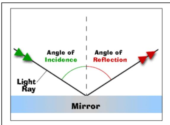
When a light wave reflects from a surface, the distance of the crest from the surface follows an absolute-value function.
