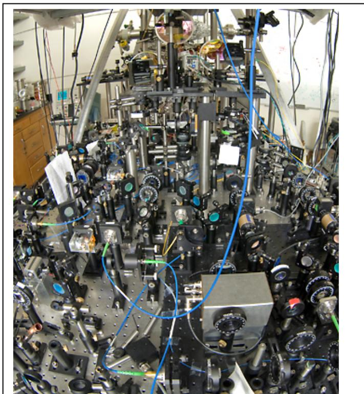
This jumble of hundreds of mirrors and lenses is used to control six beams of laser light being used in an experiment to test Einstein's theory of relativity.
