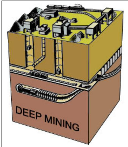
It is a very uncomfortable job working in a deep mine. As you dig deeper into the Earth, the temperature of the rock around you increases. Near Earth's surface, this rate is about 0.013 degrees Celsius per meter. The average temperature,  $T$ , in Celsius, at a particular depth,  $d$ , in meters, is given by the formula:
