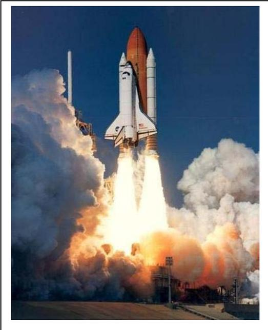
Rockets work by throwing mass out their ends to produce 'thrust', which moves the rocket forward.
