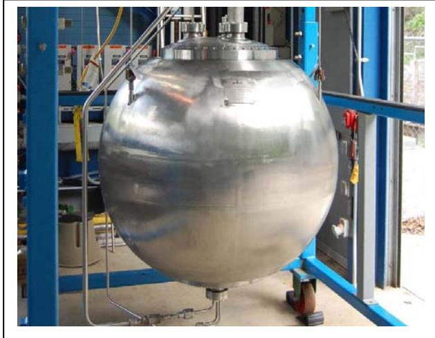
This spherical propellant tank is an important component of testing for the Altair lunar lander, an integral part of NASA's Constellation Program. It will be filled with liquid methane and extensively tested in a simulated lunar thermal environment to determine how liquid methane would react to being stored on the moon.
