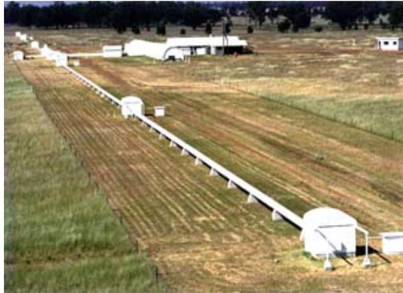
A photo of the Sydney University Stellar Interferometer (SUSI) is a long-baseline optical interferometer located approximately 20km west of the town of Narrabri in northern New South Wales, Australia. The equivalent diameter of the optical aperture for this instrument is 640 meters.
