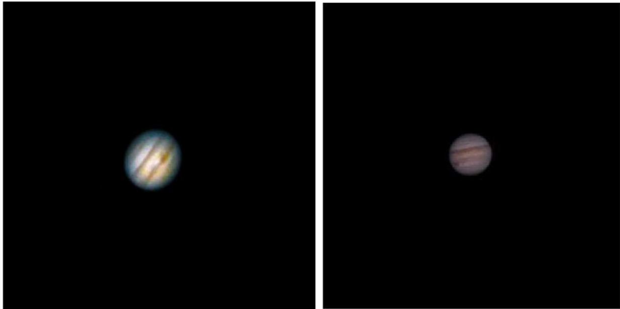
Figure 76. Jupiter – Left) 7 images stacked; Redmi 3s prime phone with adapter; 12-inch Dobsonian telescope with a 9mm Plössel eyepiece. (Credit Bhushan Karmarkar); Right) Orion 6xt 6-inch telescope with a 12 mm eyepiece shot with a Galaxy s10 and using a moon filter from a video series with the Native camera. It was edited in PIPP (cropped), stacked in Autostackert (790 frames) and post-processed in Photoshop to adjust color saturation and sharpening. (Credit Michael Armentrout).
