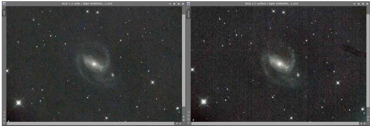
Figure 100. Faint galaxies benefit greatly from careful stacking and calibration to remove artifacts. In this comparison, the removal of vertical pattern noise and flattening of the sky background is evident. The galaxy is NGC 1097 taken with a Takahashi MT-160 (6.3-inch refractor) using a Canon EOS700D camera. (Credit Logan Nicholson)
