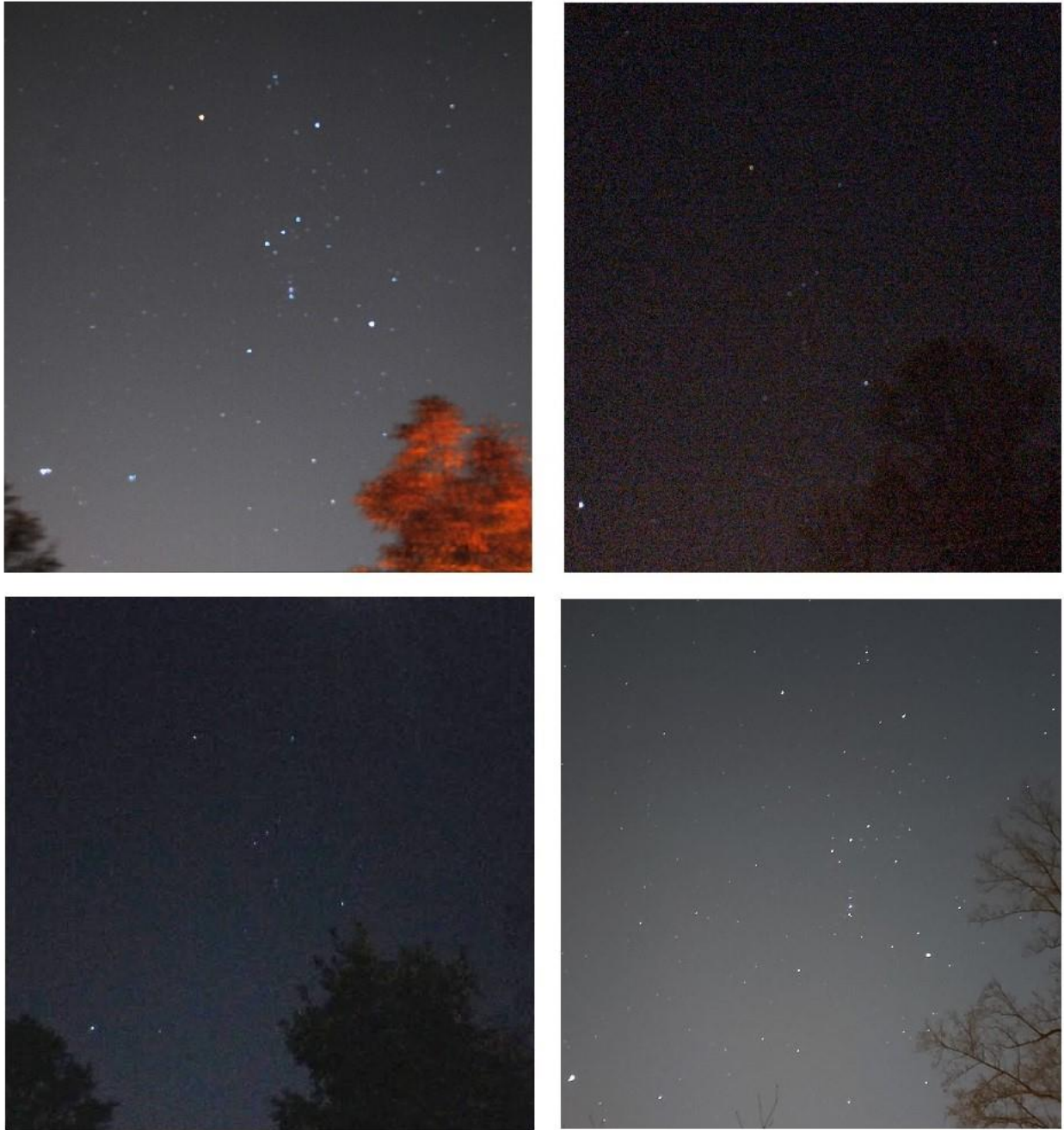
Figure 54. A variety of Orion images processed and stacked by different camera systems. Top left Nikon, Top right iPhone 6s and the Camera+ app, bottom left Galaxy S8 with Native app and Bottom right Galaxy S9+ with Native app.
