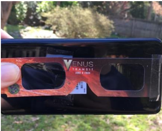
Figure 112. An example of how a proper solar filter from official solar eclipse viewing glasses can be adapted as a solar filter for a smartphone. This was taken using an old pair of NASA-approved solar viewing glasses previously used to photograph the 2004 Transit of Venus.
