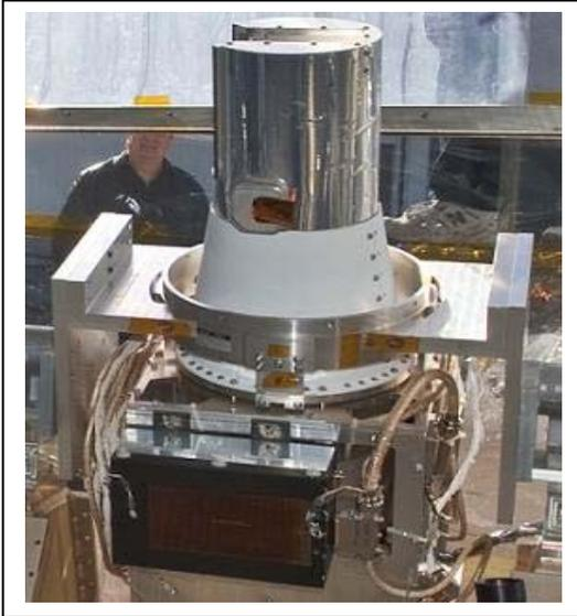
The Stratospheric Aerosol and Gas Experiment III (SAGE III), the sensor will be installed on the International Space Station (ISS) sometime in 2014. SAGE III will be using the sun and moon as light sources to measure how well the ozone layer is recovering and replenishing itself.
