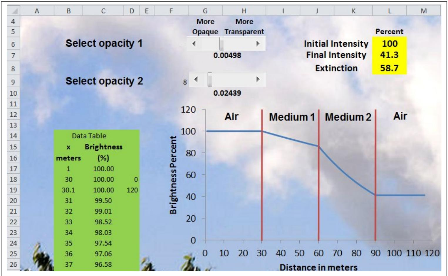
This lab allows you to examine how the change in the opacity of a material affects its ability to transmit light. The basic formula that relates opacity to transmission is given by
