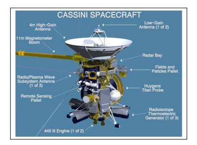
The Cassini mission is so far away from the sun that solar panels do not get enough sunlight to create solar electricity. At Saturn, the sun is nearly 90 times fainter than near Earth.
