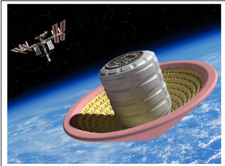
The Hypersonic Inflatable Aerodynamic Decelerator (HIAD) is a conical heat shield that can be deployed and inflated to safely reduce the speed of a payload returning to a planetary surface. The amount of 'aero breaking' it can provide depends on its surface area. Because of their lightweight design and breaking efficiency, HIAD can be made large enough to place payloads up to 40 tons on the Martian surface.
