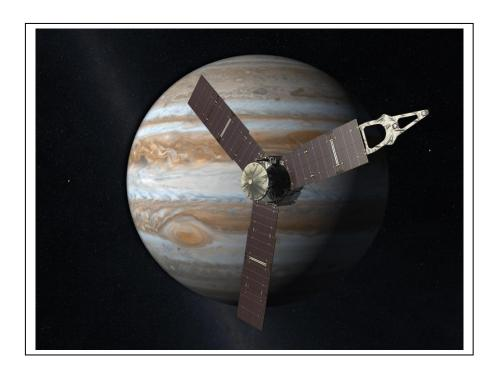
The spacecraft has three rectangular solar panels that each measure 2.7 meters wide by 8.9 meters long. At Earth, the amount of solar energy falling on the panels yields 168 watts per square meter of electrical power.
