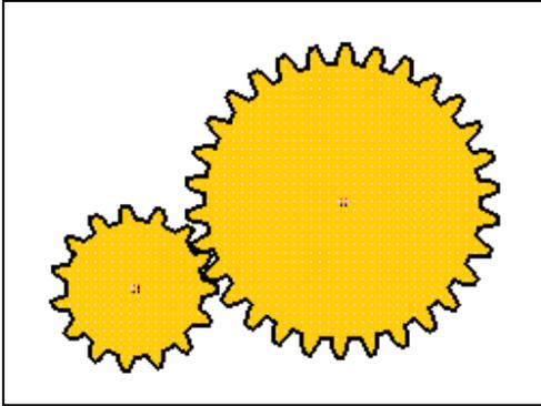
Gears are a common mechanical object used to change the rate of rotation of one shaft into a faster or slower rotation of a second shaft.
