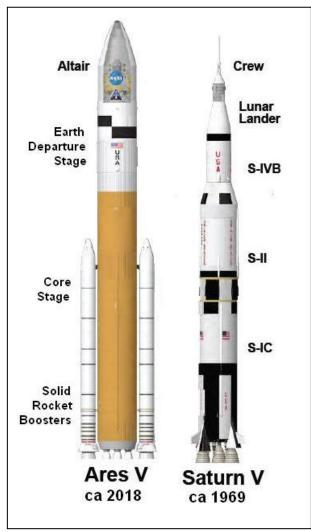
The Ares-V rocket, now being developed by NASA, will weigh 3,700 tons at lift-off, and be able to ferry 75 tons of supplies, equipment and up to 4 astronauts to the moon. As a multi-purpose launch vehicle, it will also be able to launch complex, and very heavy, scientific payloads to Mars and beyond. To do this, the rockets on the Core Stage and Solid Rocket Boosters (SRBs) deliver a combined thrust of 47 million Newtons (11 million pounds). For the rocket, let's define:
