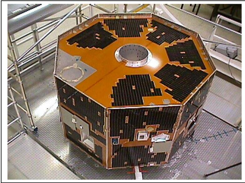
Satellites are designed to optimize the number of experiments they can carry, while at the same time keeping the mass and power requirements at a minimum. The picture shows the IMAGE satellite with the dark solar cells attached to its surface.
