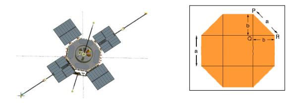
NASA's Van Allen Probes satellites are in the shape of an octagon with a thickness of 84 centimeters between the front octagonal face and the back octagonal face. An engineer needs to determine the total surface area of this 'octagonal prism' in order to create a mathematical model of how fast the satellite is warming up and cooling down as it orbits Earth.
