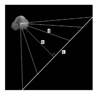
On July 4, 2005, the Deep Impact spacecraft flew by the comet Tempel-1 along a path shown in the figure to the left, at a speed of V=10 km/sec. Its closest distance to the comet was b = 500 kilometers at a time, t=0. The distance traveled along the path is given by L = Vt.
