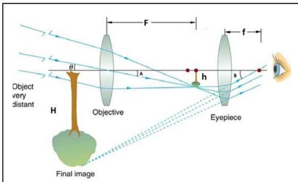
A telescope consists of an objective mirror or lens and an eyepiece. The role of the eyepiece is to change the angle,  $A$ , of the rays from the objective as they enter the eye. As the figure shows, when  $B > A$ , it appears as though the image of the tree is bigger than its actual image at the focus of the telescope objective. A simple proportion relates the image sizes to the focal lengths of the lenses:
