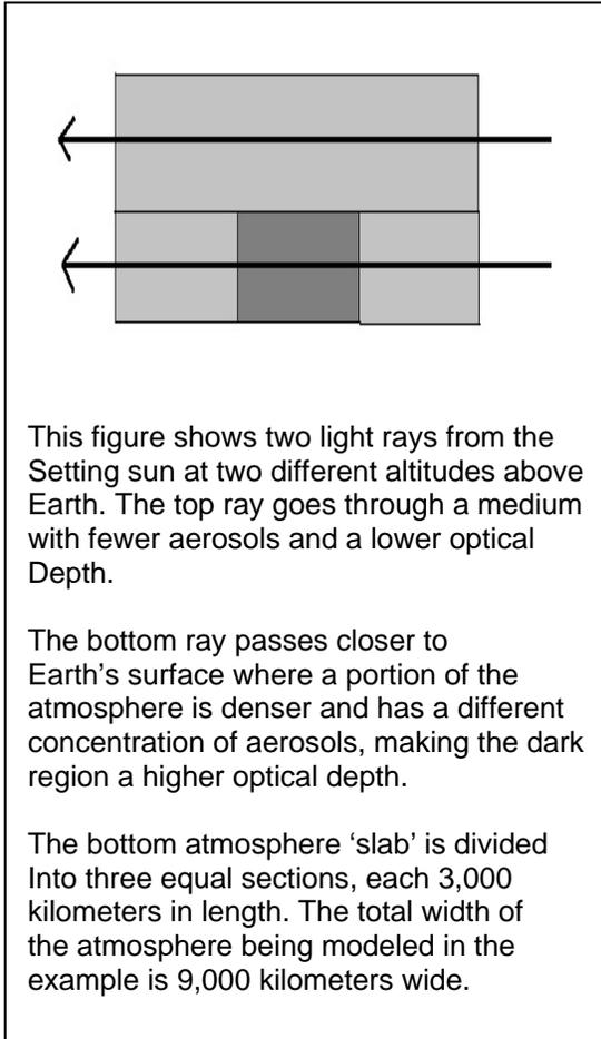
Opacity is a term used to describe the passage of light through a material, and is defined by the basic exponential formula
