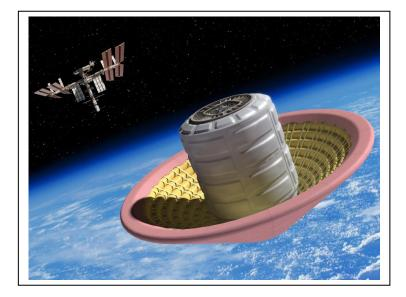
The Inflatable Hypersonic Aerodynamic Decelerator (HIAD) is a conical heat shield that can be deployed and inflated to safely reduce the speed of a payload returning to a planetary surface. The amount of 'aero breaking' it can provide depends on its surface area. Because of their lightweight design and breaking efficiency, HIAD can be made large enough to place payloads up to 40 tons on the Martian surface.
