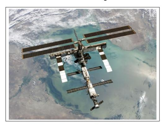
The International Space Station is a 400-ton, \$160 billion platform that supports an international team of 3-5 astronauts for tours of duty lasting up to 6 months at a time. Like all satellites that orbit close to Earth, the atmosphere causes the ISS orbit to decay steadily every day, so the ISS has to be 're-boosted' every few months to prevent it from burning up in the atmosphere.
