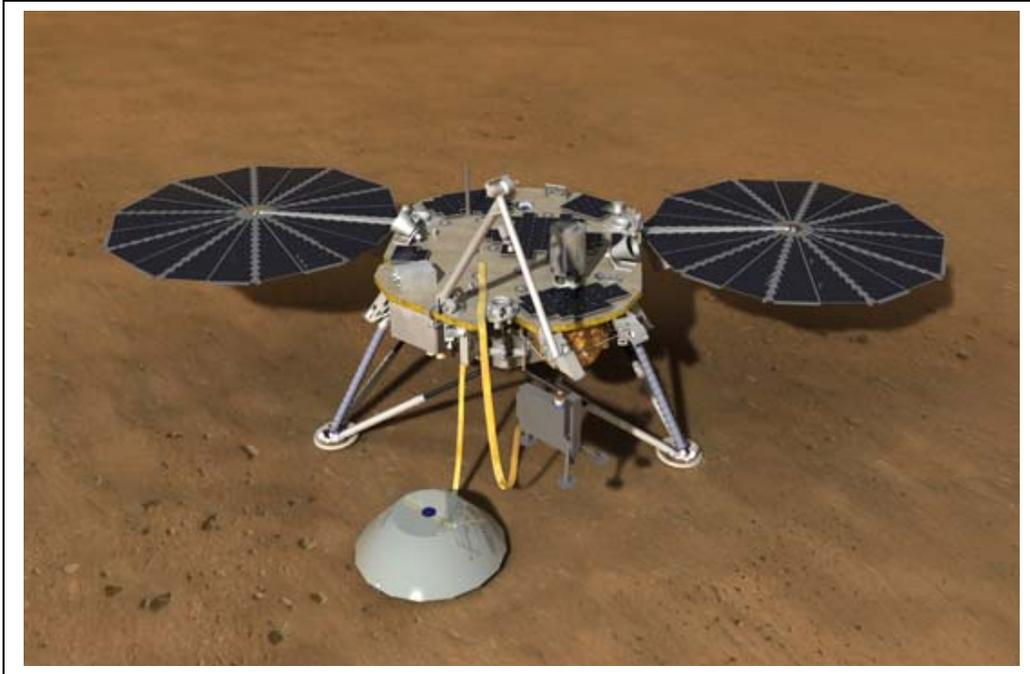
NASA's new mission to Mars called InSight will be launched in March, 2016. It will land in a region of Mars located near the equator and deploy a seismographic station and a heat probe to study the interior of Mars.
