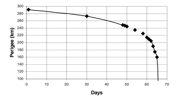
Figure 2 - Decay of the UARS satellite between July 20 and September 23, 2011.
